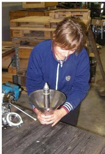
Pict. 16: Remove the funnel by sliding it downwards over the cone
