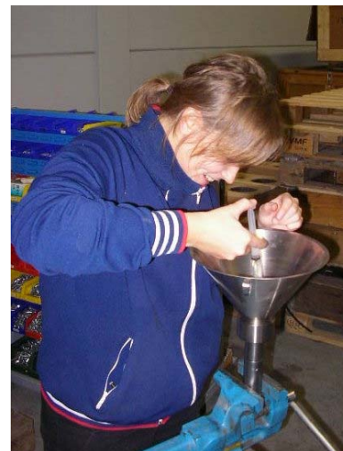
Pict. 3: Fill the housing of the pore pressure sensor with de-aired glycerine
