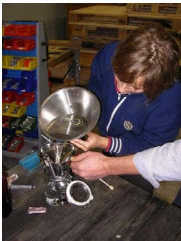
Pict. 15: Pour the saturation fluid gently back into the airtight container
