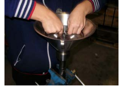
Pict. 11: Maneuver the filter onto the cone tip. Make sure that everything remains submerged
