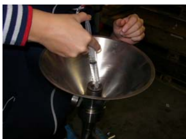
Pict. 4: Fill the housing of the pore pressure sensor with de-aired glycerine layer by layer
