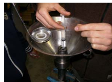
Pict. 6: Remove last remaining air bubbles and bring in the filter using the ladle
