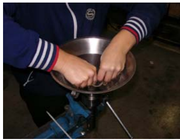
Pict. 13: Flip the inside of the condom outwards and back and slide it over the cone
