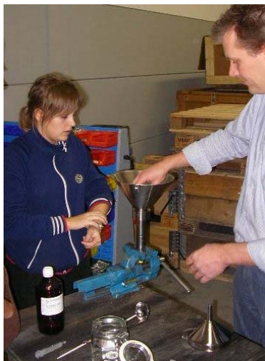
Pict. 1: Cone top-up in bench vice and saturation funnel in place
