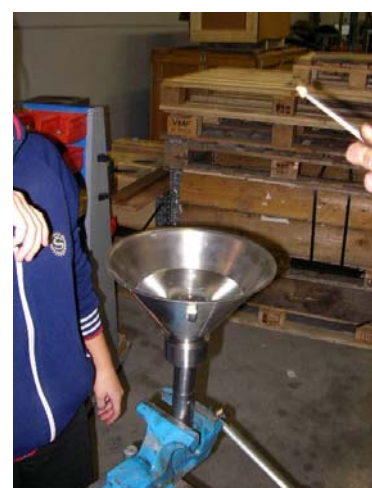
Pict. 7: Cone and funnel filled with de-aired glycerine and saturated filter
