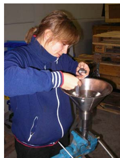
Pict. 8: Fill the syringe with glycerine from the funnel and keep the cone tip handy
