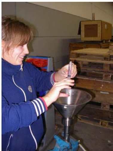
Pict. 2: Fill the syringe with de-aired glycerine and force remaining air out
