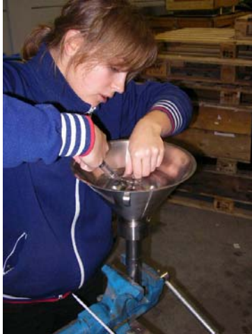
Pict. 9: Squeeze the glycerine through the hole in the cone tip whilst submerged
