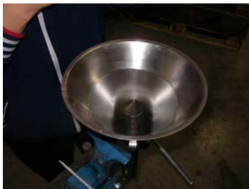
Pict. 12: Screw the cone tip and filter onto the cone
