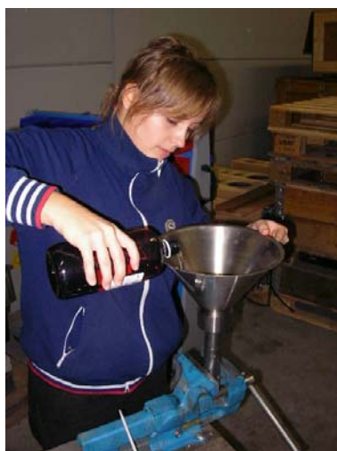
Pict. 5: Fill the saturation funnel with de-aired glycerine
