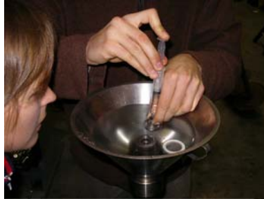
Pict. 10: Make sure there are no air bubbles left in the cone tip
