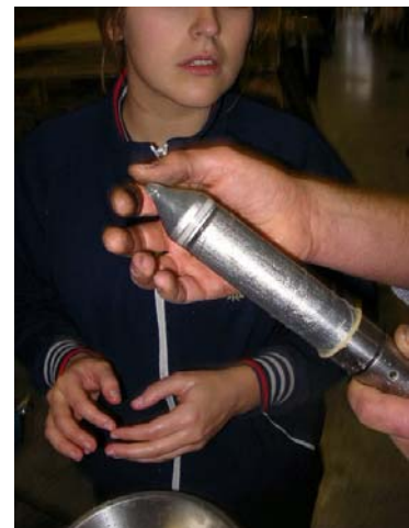
Pict. 17: Adjust the condom such that it causes no over- or underpressure on the filter. The piezocone is now ready for CPTU
